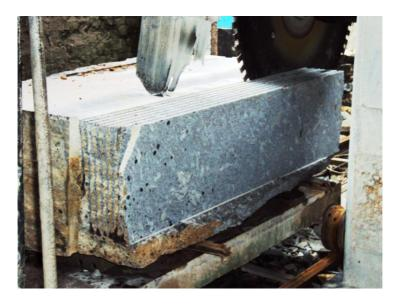
for quarrying as against the traditional rock blasting to minimize the impact on the environment as well as to prevent the quarried stones developing hair cracks that may open up subsequently.
